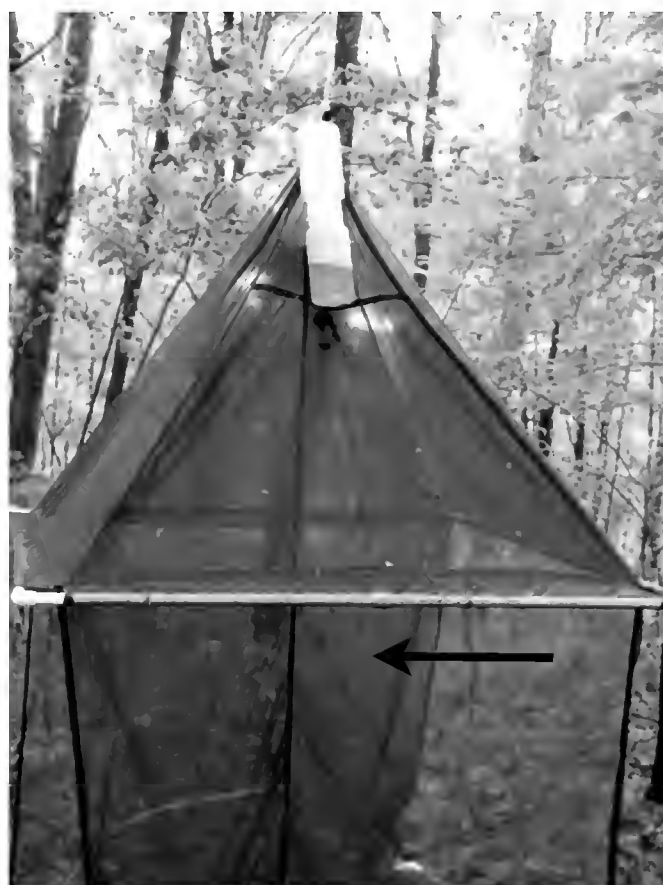
(figure 2.) Lower collection vial where beetles that “hit and drop” are collected.
